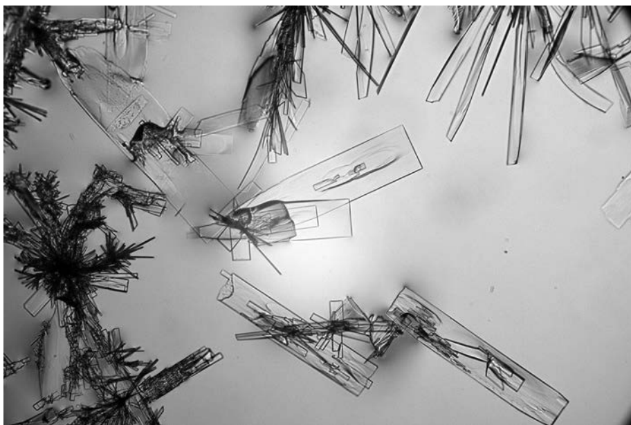
Figure III. "Paddlewheel and rosette of blade" shaped crystal observed during a microcrystalline test for mephedrone [34]
